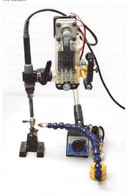
Operator's-eye-view of the soldering station. An old "third hand" clamp is repurposed as a saddle to hold connectors while the wire is positioned from left. Solder is fed from in front and the iron descends from above, on command.
