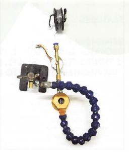
Solder feeder made from a small stepper motor and some 3D printer spare parts. A brass pinion drives the solder wire by friction, within a brass tube glued to the motor's mounting plate. The solder is fed through a flexible arm intended for milling machine coolant; the tip has an old 3D printer nozzle drilled out to feed the solder.
