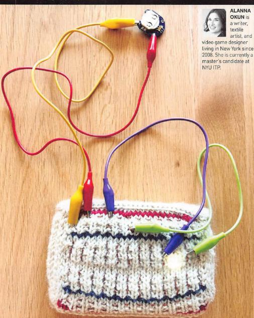
The solderless breadboard is a cornerstone of electronics education and prototyping — a rectangular waffle that conducts electricity in configurations of columns and rows, for testing and determining where wires and components should connect to one another in a circuit, before more permanent measures like soldering.
